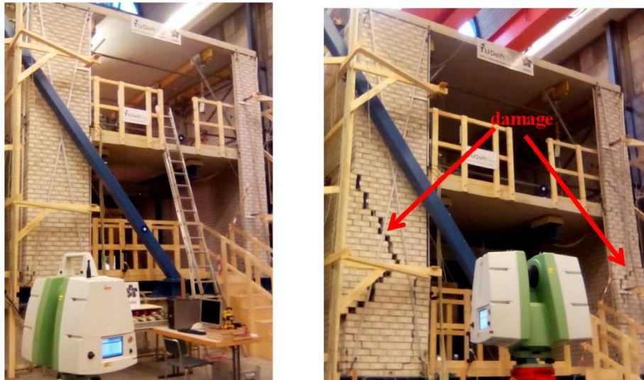
Figure 1: Lab induced damage measured by Terrestrial Laser Scanning
